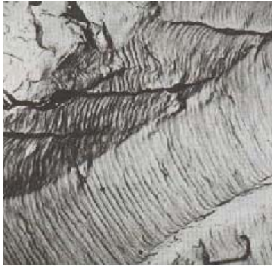
Figure 2 Example of Beachmarks and striations found in fatigue fracture
